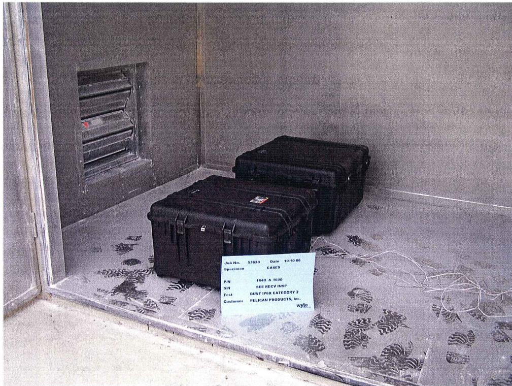
Photograph 1 Dust Test Setup (Tested with other Pelican Product Items)
