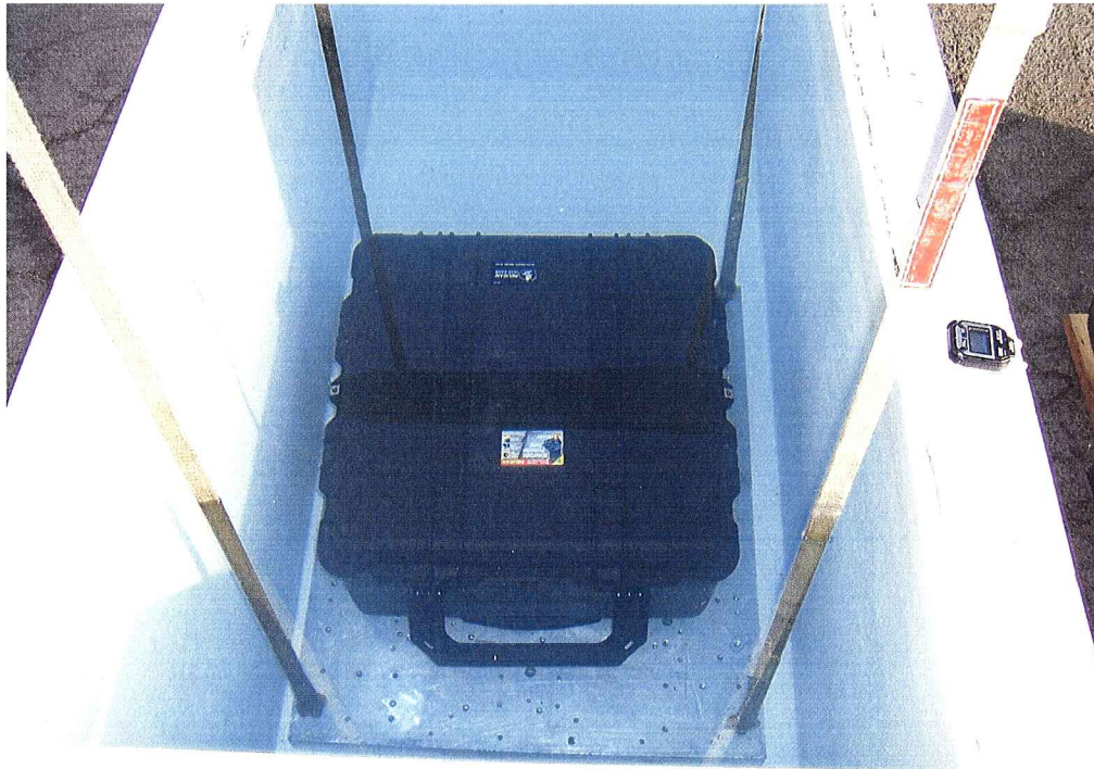
Photograph 4 Immersion Test Setup
