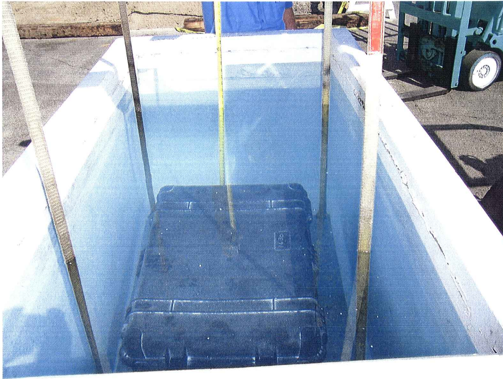
Photograph 3 Immersion Test Setup
